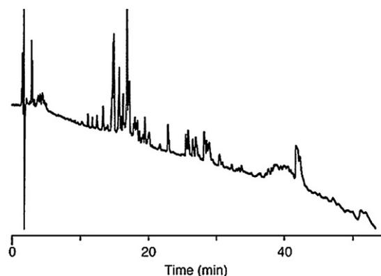
**Fig. 8.** Separation of tryptic digest of BSA. Column: 200T-MAS-AA, 200  $\mu$ m ID  $\times$  22 cm. Mobile phase: A: water (0.2% HCO<sub>2</sub>H); B: ACN; linear gradient in 60 min, 90–10% B;  $\lambda$ : 220 nm, injection volume: 50 nl. Reproduced with permission from [62].
