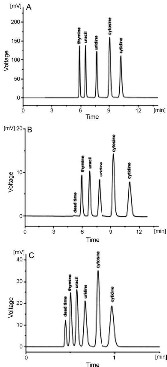
**Fig. 5.** Separations of pyrimidines and purines on two HILIC columns. Conditions: (a) commercial ZIC-pHILIC column 150 mm  $\times$  1.0 mm ID (3.5  $\mu\text{m}$ ); (b and c), poly(SP<sub>V</sub>-co-MBA) column 300 mm  $\times$  100  $\mu\text{m}$  ID; mobile phase, ACN/H<sub>2</sub>O (80:20, v/v) containing 25 mM ammonium formate, pH 6.4; wavelength, 254 nm. Backpressure: a, 50 bar; b, 20 bar; c, 180 bar.
