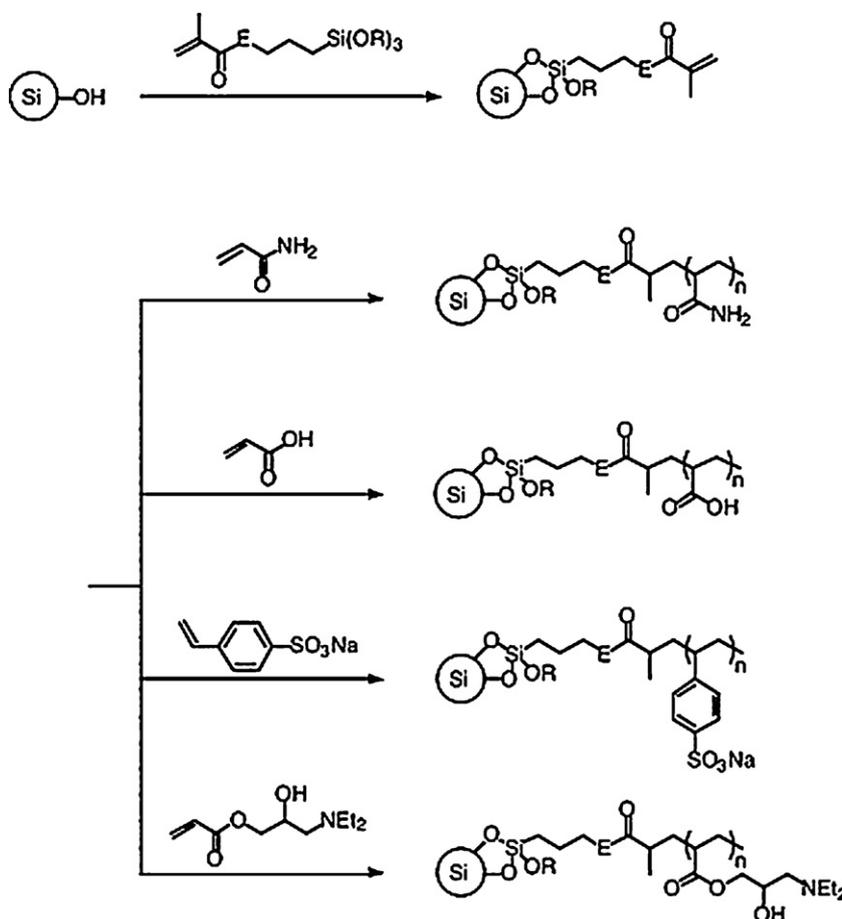
Fig. 1. Synthetic scheme of the polymer-coated monolithic silica columns [64].
