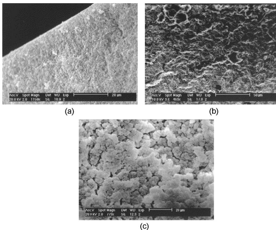
**Fig. 4.** Effects of ammonium sulphate concentration on the morphology of poly(DMAA–PDA–VSA) monoliths ( $T = 29\%$ ,  $C = 52\%$ ), prepared in the presence of (a) no, (b) 20 mg/ml, and (c) 120 mg/ml ammonium sulphate in 50 mM phosphate buffer, pH 7. Reproduced with permission from [82].
